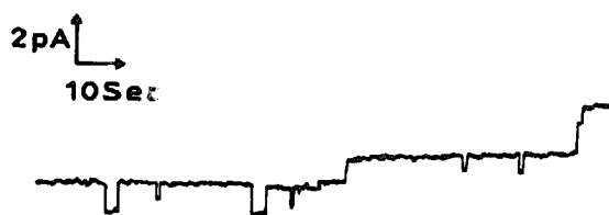
Fig. 1. Current steps induced by \alpha -LaTx in a lipid bilayer made of egg-phosphatidylcholine and cholesterol. Toxin was added to the cis side of the membrane (final concn. 6 \cdot 10^{-10} \text{ M} ) interposed between symmetrical solutions of 100 mM KCl buffered at pH 7.5 with 10 mM Tris-HCl. A 40 mV positive potential was applied to the trans side, while the cis side was at virtual ground.
